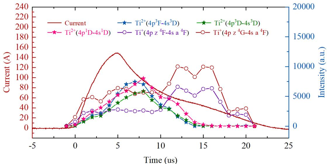
Fig. 1 Time evolution of discharge current and emission intensities of  $\text{Ti}^+$  and  $\text{Ti}^{2+}$ .
