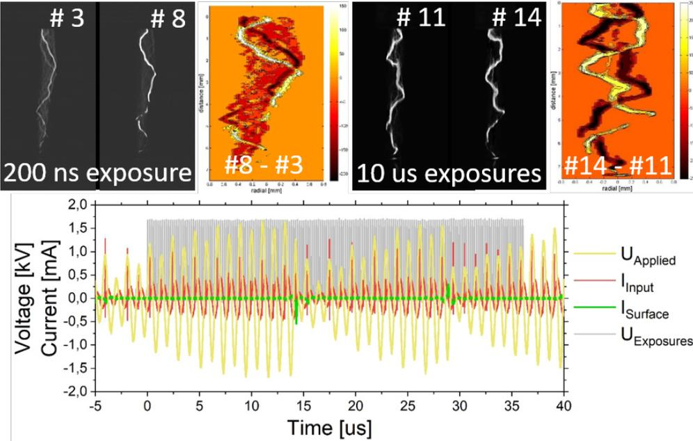
Fig 1: Images of guided streamer formation within two voltage cycles and an image subtraction (200 ns and 10 us exposures), electrical signal of correlated voltage, input and surface current
