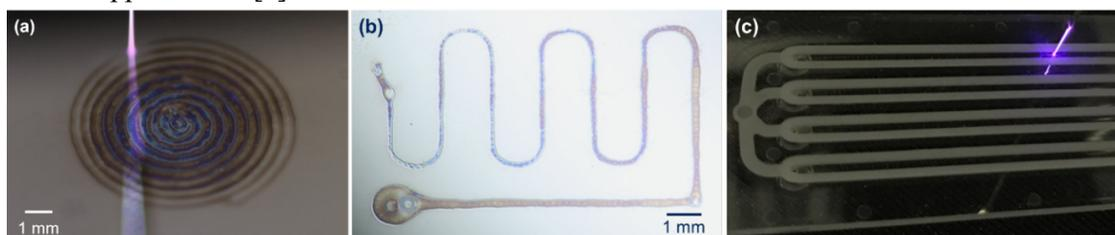
Fig. 1 Deposition of plasma-polymerized micropatterns on silicon wafer (a-b) and a polystyrene microfluidic chip (c), using SurfAP<sup>3</sup>® technology. The microplasma discharge is seen in (a) and (c).
