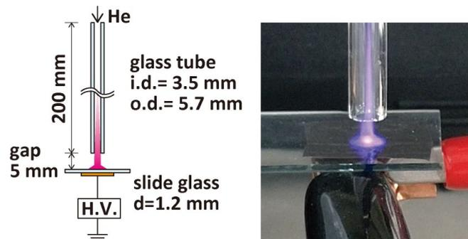
Fig. 1 Schematic illustration of the experimental setup for launching plasma bullets from the surface of a glass plate, and overview of the consequent APPJ.
