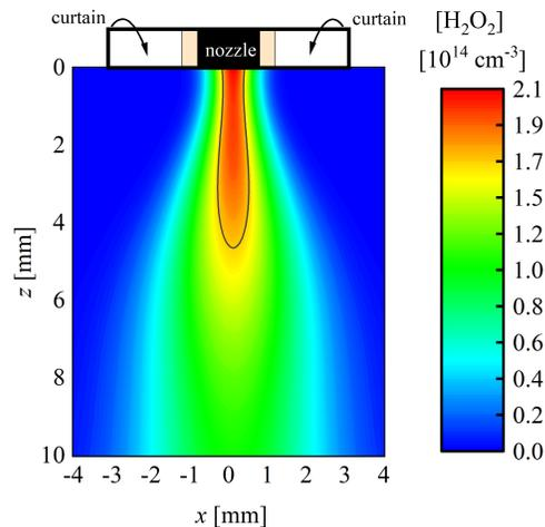
Fig. 1 A lateral contour plot of  $\text{H}_2\text{O}_2$  densities in the effluent of the kINPen plasma jet.
