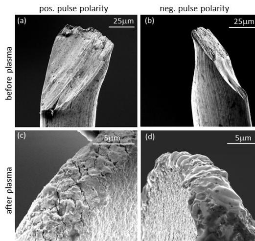
Fig. 1 SEM images before (top row) and after (bottom row) ns plasma ignition in water with positive polarity (left column) and negative polarity (right column) [1].
