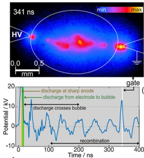
Fig. 1 Discharges in an Ar bubble in deionized water. Applied voltage ramp rate  $\sim 3$  kV/ns, maximum 20 kV.
