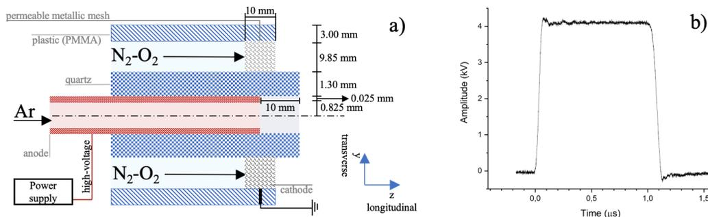
Figure: a) Cross-sectional scheme of the co-axial APMPJ reactor, b) Applied high-voltage pulse
