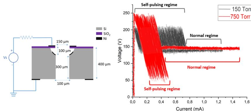
Figure 1: a) Design of the microreactor, b) V-I characteristics in He with a 1 M $\Omega$  ballast resistor.
