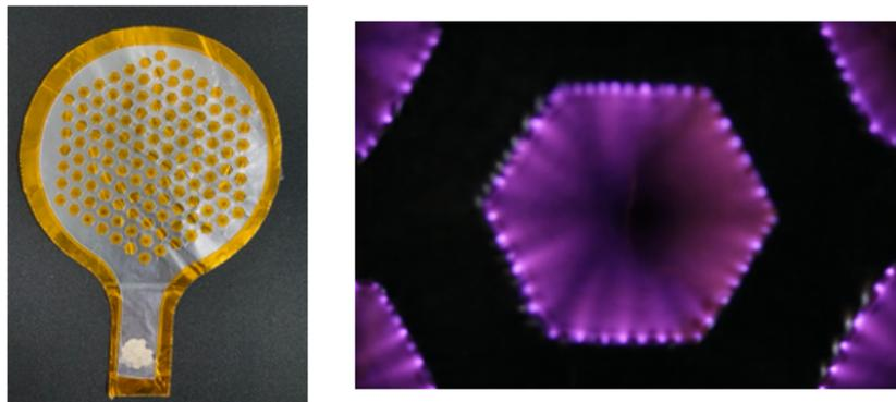
Fig. 1 Left: Prototype of surface dielectric barrier discharge electrode. Right: Close up of plasma generated inside of hexagonal lattice.
